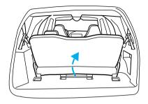
5. While pulling up on the release bar, lift the seat up and out of the floor tubs and roll seat rearward.
